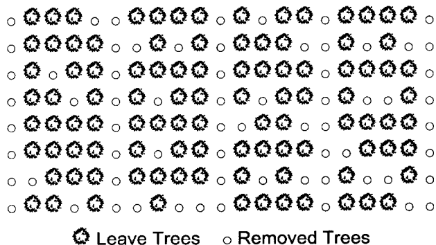
Figure 6: Typical pattern for a combination thinning in a pine plantation.
